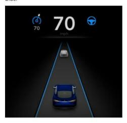
Note: To initiate Autosteer, you must be driving at least 18 mph (30 km/h) on a roadway with visible lane markings. If a vehicle is detected ahead of you, you can initiate Autosteer at any speed, even when stationary.
