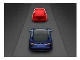
Warnings cancel automatically when the risk of a collision has been reduced (for example, you have decelerated or stopped Model S, or a vehicle in front has moved out of your driving path).
